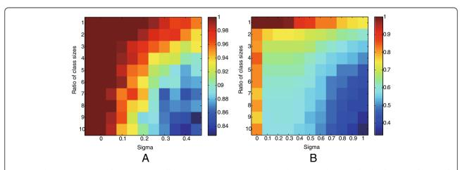
Figure 1 Clustering accuracy of OTCC (A) and Affinity Propagation (B) on simulated data sets with various levels of noise and ratios of class sizes. "Sigma" is the standard variation of noise distribution.
